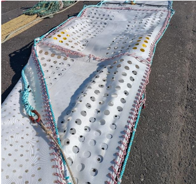
Figure 14. Image of FloMo showing 55mm apertures on top sheets and 20mm apertures on bottom sheets.
